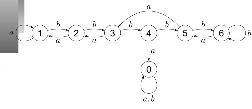
This 0-monotonic automaton is the first in Ananichev's series that yields the lower bound  $SAS(n) \ge n + \left\lfloor \frac{n}{2} \right\rfloor - 2$ . It has 7 states and its shortest reset word is  $a^4b^3a$  of length  $7 + \left\lfloor \frac{7}{2} \right\rfloor - 2 = 8$ .
