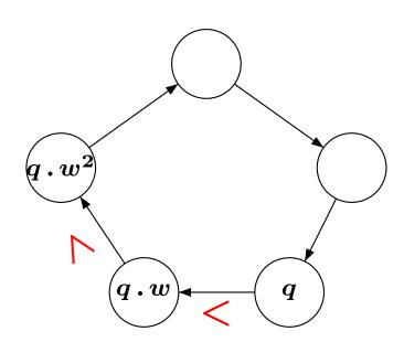
A DFA  $\mathscr{A} = \langle Q, \Sigma, \delta \rangle$  is *monotonic* if Q admits a linear order  $\leq$  such that, for  $a \in \Sigma$ , the transformation  $\delta(\Box, a)$  of Q preserves  $\leq$ :
