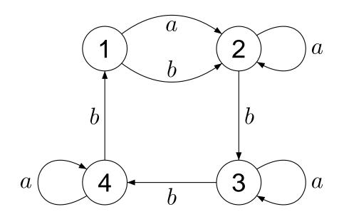
A reset sequence of actions is *abbbabba*. Applying it at any state brings the automaton to the state 2.
