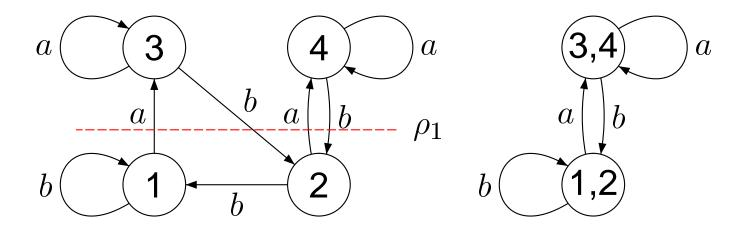
Endowing Q with the order  $\leq_1$  such that  $1 <_1 2$  and  $3 <_1 4$ , we see that the automaton is  $\rho_1$ -monotonic. If we order  $Q/\rho_1$  by letting  $\{1,2\} <_2 \{3,4\}$ , the quotient automaton becomes monotonic.
