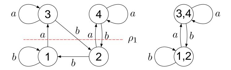
Endowing Q with the order  $\leq_1$  such that  $1 <_1 2$  and  $3 <_1 4$ , we see that the automaton is  $\rho_1$ -monotonic.
